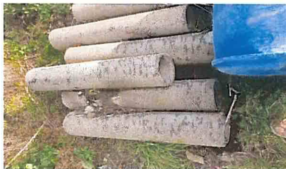
Photographs; Showing the HDPE water pipe and 6-inch concrete sleeving used to weigh pipe down. Pipe and sleeving have been in place 25 years and are buried underneath mud and silt.
