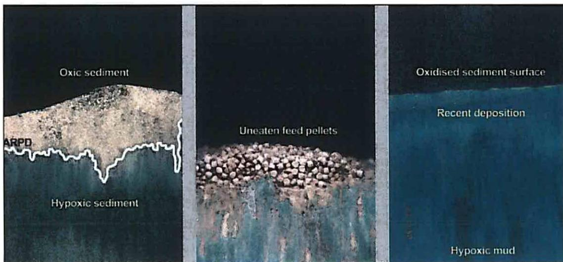
Figure 2.3: Typical sediment profile images with examples of features relevant to aquaculture operations
