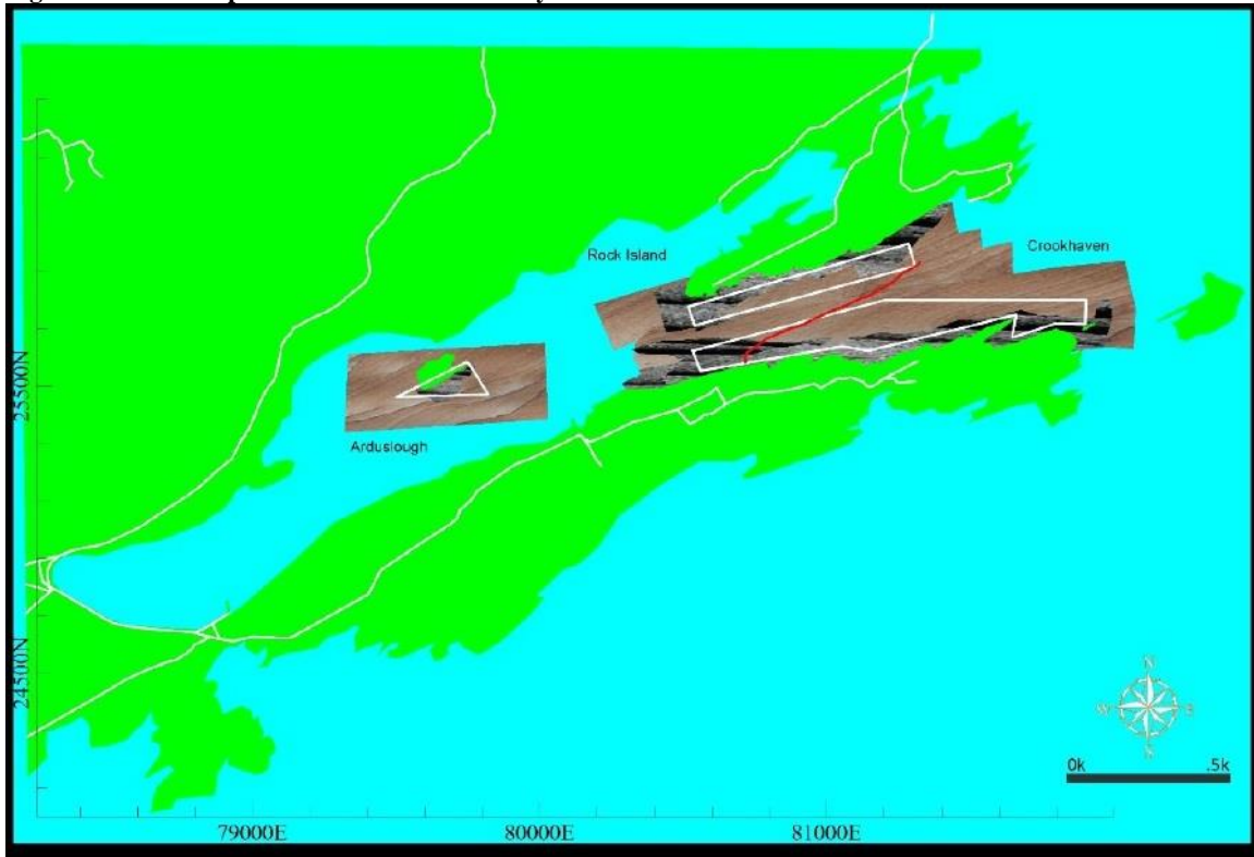
Figure 18 Subsea Pipeline Location Identified by Sidescan Sonar
